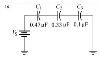
What is the capacitance of the circuit shown in the given circuit?
