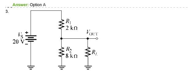
If the load in the given circit is 120  $k^{\Omega}$  , what is the loaded output voltage?
