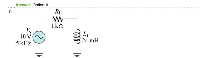
The voltage dropped across the resistor in the circuit in the given circuit is approximately equal to
