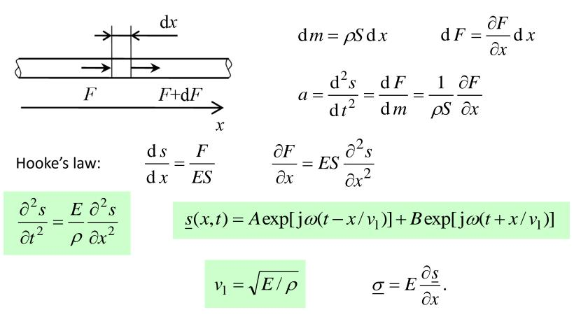
Here s is displacement;  $\sigma$  is stress.
