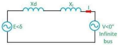
Equivalent diagram of synchronous machine connected to an infinite bus through a transmission line of series reactance  $X_1$  is shown below:
