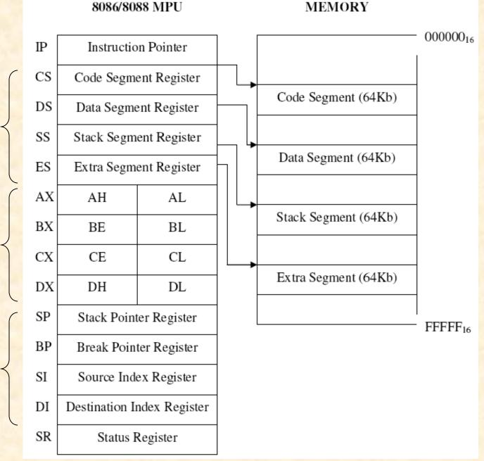
**Data segment** (DS) is a 16-bit register containing address of 64KB segment with program data. By default, the processor assumes that all data referenced by general registers (AX, BX, CX, DX) and index register (SI, DI) is located in the data segment. DS register can be changed directly using POP and LDS instructions.
