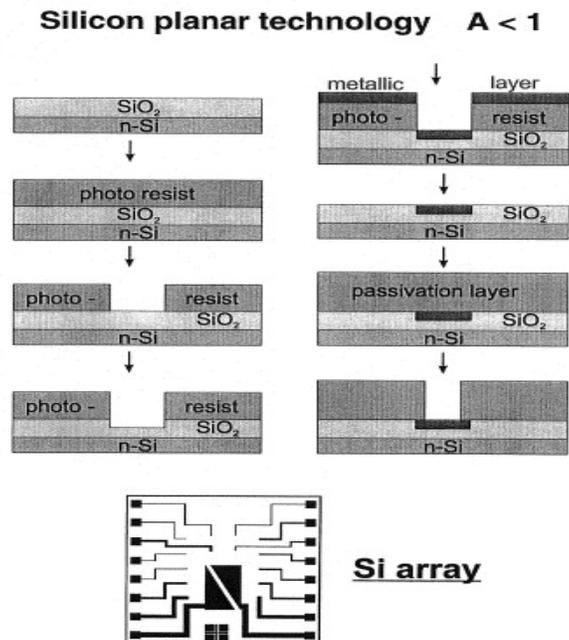
Photo resists are of two types: negative & positive. Materials which are rendered less soluble in a developer solution by illumination yield a negative pattern of the mask and are called negative photo resists.
