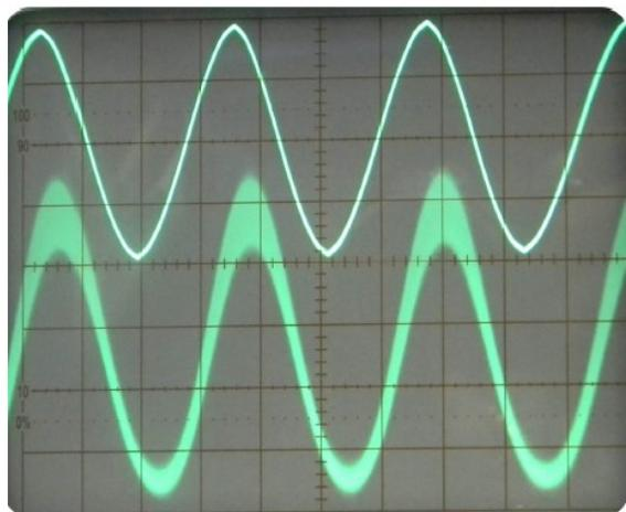
**Diode Detector output**
