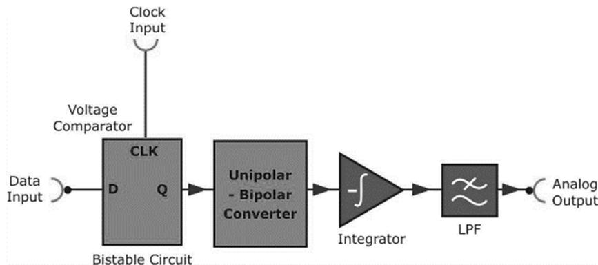
and quantized as with PCM. If the sample currently being coded is above the previous sample, then a binary bit is set to logic '1'. If the sample is lower than the
