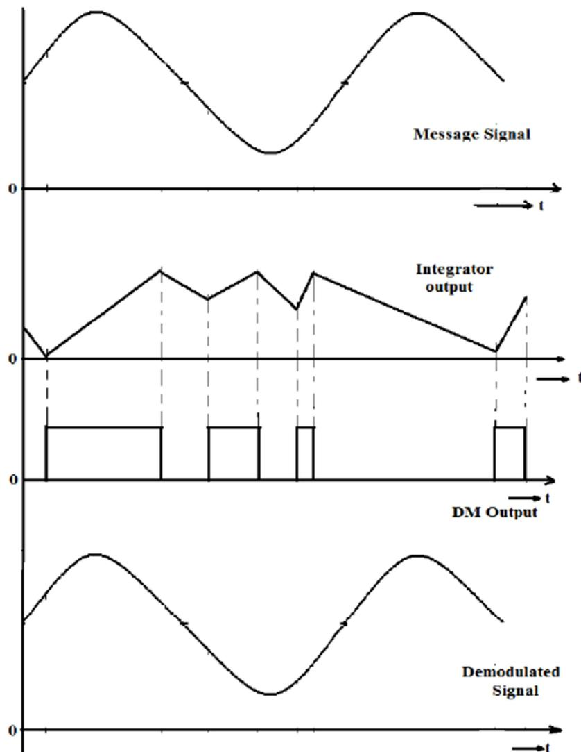
Waveforms of Delta Modulation & Demodulation
