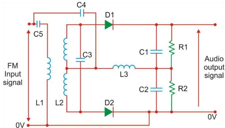
Figure 3 Foster –Seelay Detector
