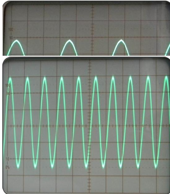
**Step 4** 1 MHz Crystal Oscillator Block generates a sine wave of 1 MHz frequency and 120mV pp amplitude approx, which is used as a carrier input to Balance Modulator and Band Pass Filter Circuit 1. Observe the carrier waveform at output test point on Oscilloscope. [CH1(Y) – 10mV; Time base – 1 uS]
