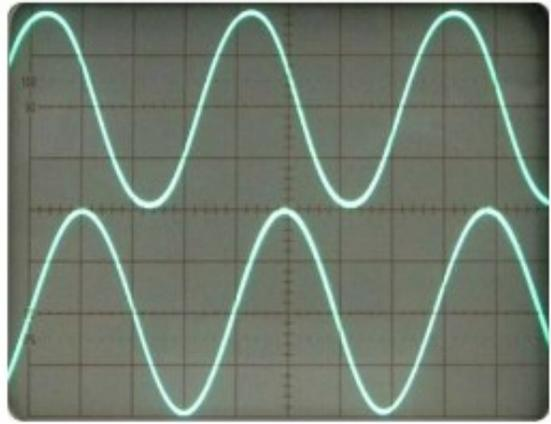
**Step 15** Connect the **Sample & Hold output** to the input of low pass filter Observe the output of the Low pass filter TP (12) together with Modulation signal input TP (2).
