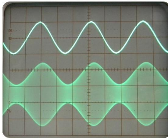
Since Scientech 2201 TX output select switch is in the ANT position, the AM signal at the output is fed to the transmitter's antenna. Prove this by touching Scientech 2201's antenna, and nothing that the loading caused by your hand reduces the amplitude of the AM waveform at the output.
