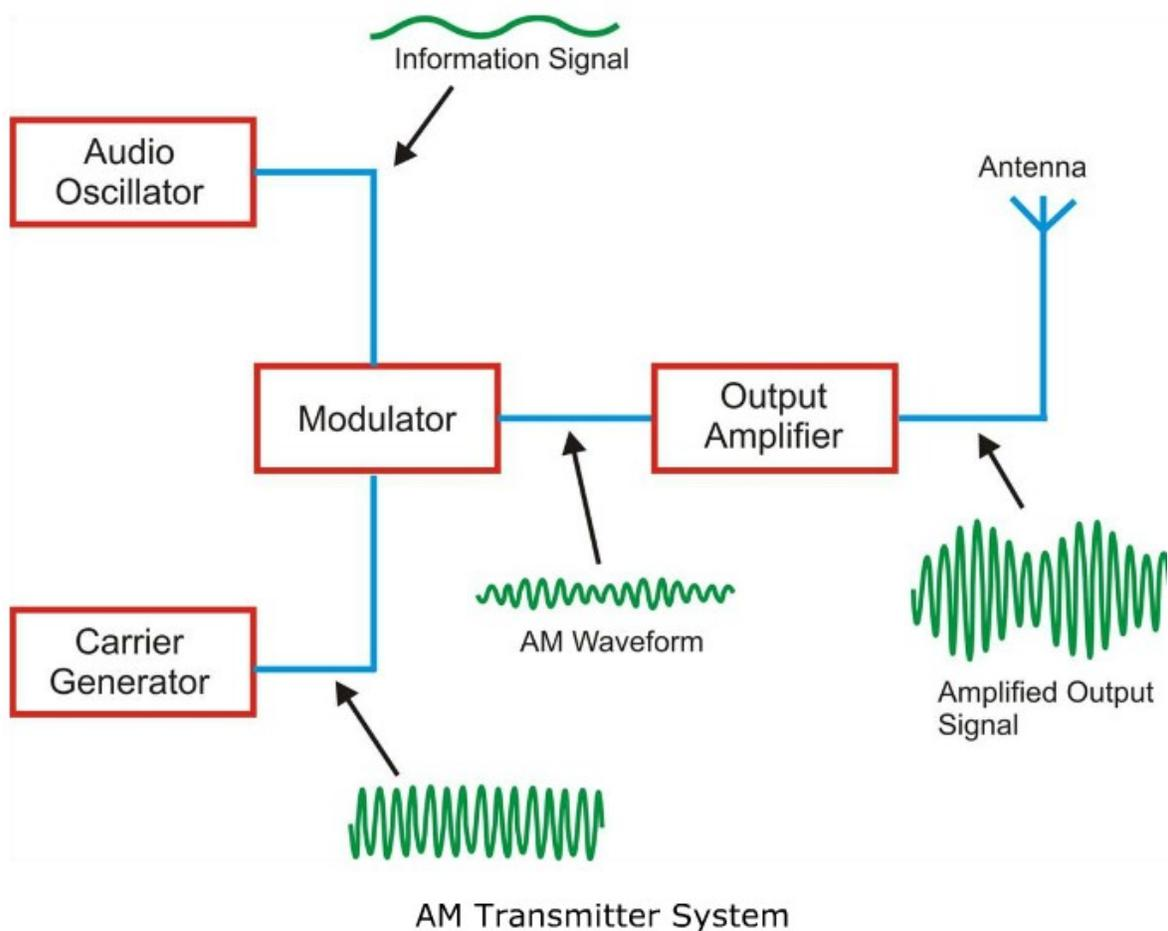
Amplitude Modulation is the process of changing the amplitude of a relatively high frequency carrier signal in proportion with the instantaneous value of the modulating signal. The general equation of Amplitude Modulated signal is given by
