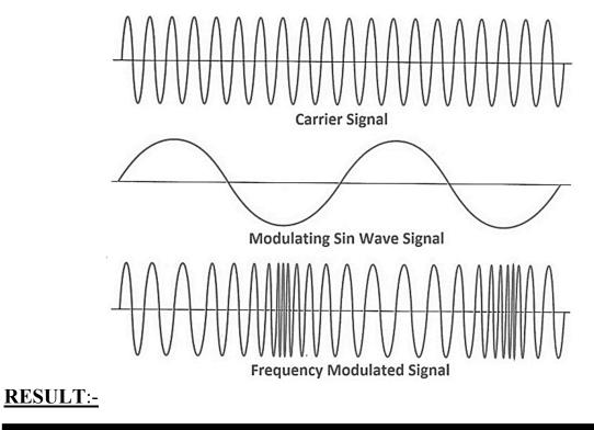
Frequency modulated wave using VCO is obtained on CRO and mf is calculated.
