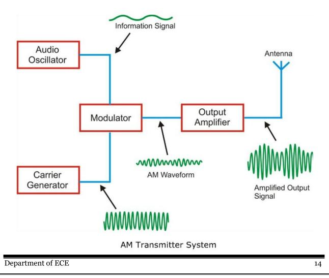
Amplitude Modulation is the process of changing the amplitude of a relatively high frequency carrier signal in proportion with the instantaneous value of the modulating signal. The general equation of Amplitude Modulated signal is given by  $s(t) = A_c (1 + x(t)) \cos \omega_c t$
