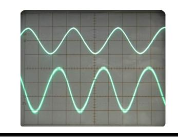
[CH1(Y) - 0.5V; CH2(X) - 0.2V Time base - 0.1 mS]TABULATION:- [CH1(Y) - 1V; CH2(X) - 2V Time base - 0.1 mS]
