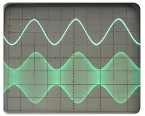
Step 6 To determine the depth of modulation, measure the maximum amplitude  $(V_{max})$  and the minimum amplitude  $(V_{min})$  of the AM waveform, and use the following formula:
