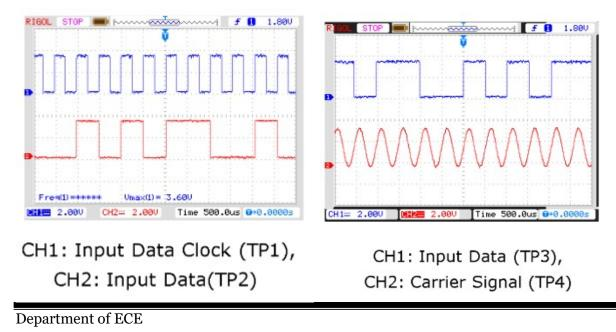
(balanced modulator) The resulting output is the ASK wave. This is illustrated in figure modulation causes a shift of the baseband signal spectrum. The ASK signal which is basically the product of the binary sequence and the carrier signal.
