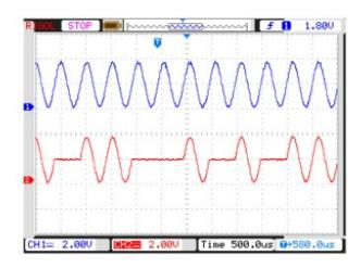
CH1: Carrier signal (TP4), CH2: ASK Output (TP5)
