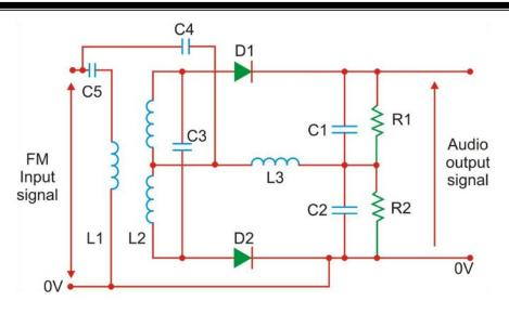
Figure 3 Foster –Seelay Detector
