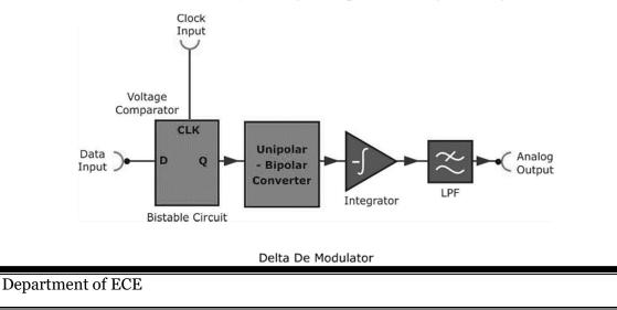
and quantized as with PCM. If the sample currently being coded is above the previous sample, then a binary bit is set to logic '1'. If the sample is lower than the
