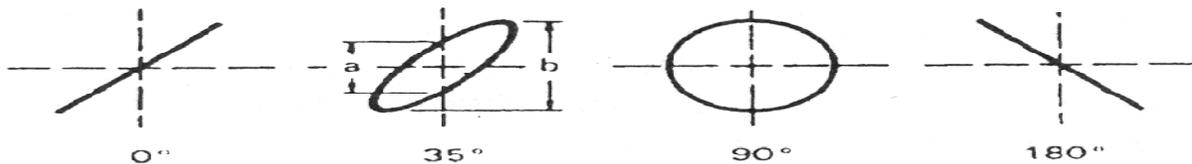
Fig: 6 Phase measurement using CRO
