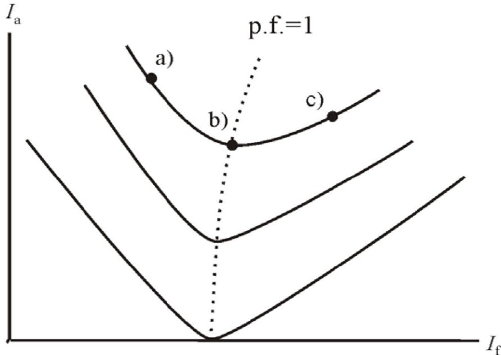
Figure 5. Synchronous motor V-curves.
