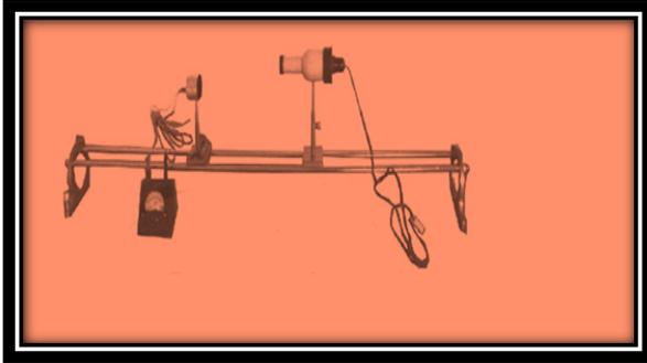
**Procedure:** The optical bench contains two uprights and carries the electric bulb and other carries a photovoltaic cell. The two terminal of photovoltaic cell is connected to ammeter.
