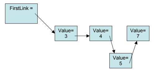
In Chapter 9 we noted how a linked list could be developed using a pair of classes. The class Link is used to store an individual link value:
