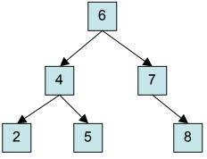
Inserting a value into or removing a value from a binary search tree requires only a traversal from the top to bottom, which is much faster than examining every elements as is required by a vector or linked list.
