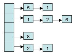
Notice that the elements do not appear to be ordered by their values in any particular way. Assuming that the lists do not become too long, insertions and removals from a hash table can be very fast. In order to assure good performance one trick is to increase the size of the table when a threshold of values have been reached (for example, when the number of elements is three times the size of the table).
