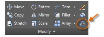
Select the object (1), specify the offset distance, and click to indicate on which side of the original that you want the result (2). Here is an example of offsetting a polyline.
