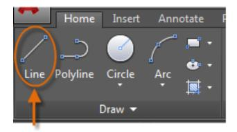
Alternatively, you can type **LINE** or just **L** in the Command window, and then press Enter or the Spacebar.
