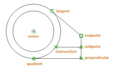
Object snaps become available during a command whenever AutoCAD prompts you to specify a point. For example, if you start a new line and move your cursor near the endpoint of an existing line, the cursor will automatically snap to it.
