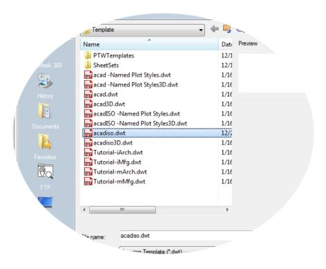
The "Tutorial" template files in the list are examples of the architectural or mechanical design templates using both imperial (i) and metric (m) measurements. You might want to experiment with them.
