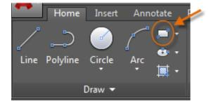
Simply click two diagonal points for the rectangle as illustrated. If you use this method, turn on grid snap (F9) for precision.
