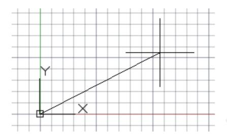
After you specify the next point, the **LINE** command automatically repeats itself, and it keeps prompting you for additional points. Press Enter or the Spacebar to end the sequence.
