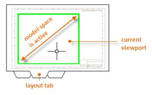
In a layout, when model space is active, you can pan and zoom, and anything else that you could do on the Model tab. For example, let's say that you created a backyard deck design in model space, and now you want to lay out and print your design from a layout tab.
