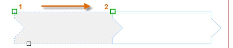
Next, to add the 1/8" space between the tiles, click the Move tool or enter **M** in the Command window. The **MOVE** command is similar to the **COPY** command. Select the newly copied tile, and press Enter or the Spacebar. As before, click anywhere in the drawing area and move your cursor to the right. Enter 1/8 or .125 for the distance.
