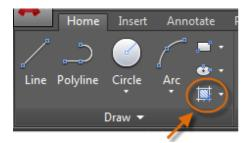
When you start the **HATCH** command, the ribbon temporarily displays the Hatch Creation tab. On this tab, you can choose from over 70 industry-standard imperial and ISO hatch patterns along with many specialized options.
