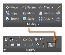
The draw order options that are listed include sending all hatches to the back, all text to the front, and so on.
