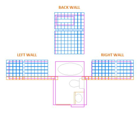
You can save a lot of work by taking advantage of the symmetry between the left and right walls. All you need to do is create the tiles on one wall and then mirror the wall across the center of the room.
