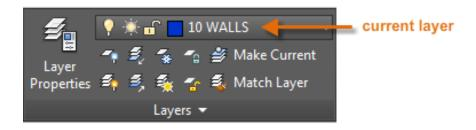
Occasionally, check to make sure that the objects you create will be on the correct layer. It's easy to forget to do this, but it's also easy to set. Click the drop-down arrow to display a list of layers, and then click a layer on the list to make it the current layer. You can also click on any layer setting icon in the list to change its setting.
