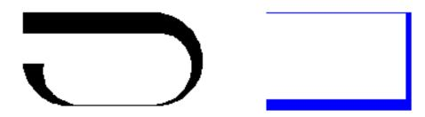
A fast way to create closed rectangular polylines is to use the **RECTANG** command (enter **REC** in the Command window).
