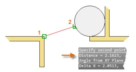
The number of decimal places and unit style displayed in the result is controlled by the **UNITS** command.
