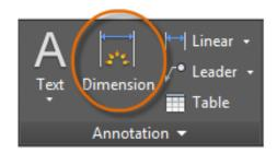
The following illustration demonstrates one method for using the **DIM** command. Once you start the command, press Enter or the Spacebar, select the line (1), and then click the location of the dimension line (2).
