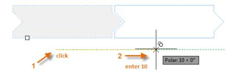
Next, move your cursor to the right, relying on the polar tracking angle to keep the direction horizontal, and then enter 10 for the distance. Press Enter or the Spacebar a second time to end the command.
