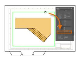
6. In the Properties palette, specify a standard scale of 1/4" = 1'-0" from the drop-down list. This action scales your view of model space precisely to the D-size drawing. You should also set the Display Locked property from No to Yes, which will prevent any unintentional display changes to the view.
