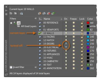
As indicated, layer 10 WALLS is the *current layer*. All new objects are automatically placed on that layer. In the list of layers, the green check next to layer 10 WALLS indicates that it is the current layer.
