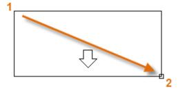
The exact size of the text box is not that important. After you specify the text box, the In-Place Editor is displayed and you can easily change the length and width of the note before, during, or after typing the text.
