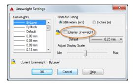
Regardless of the display setting, lineweights will always be printed at the correct scale.
