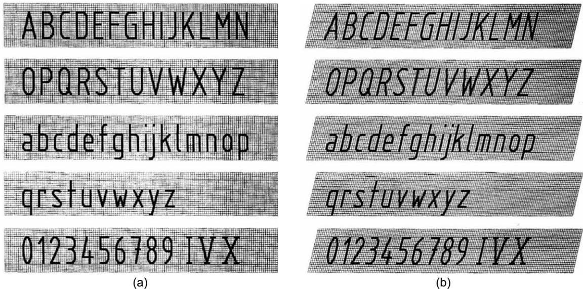
Fig. 2.3 Lettering A (a) Single-stroke vertical letters (b) Single-stroke inclined letters
