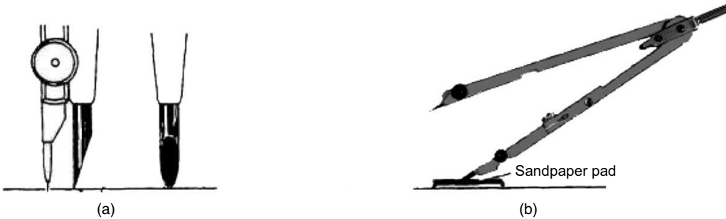
Fig. 1.11 (a) Setting length of needle point (b) Preparing pencil lead
