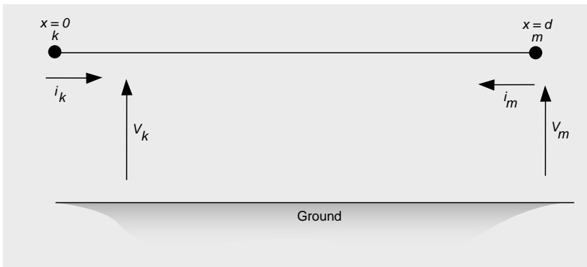
Figure 10.39 Transmission line with earth return
