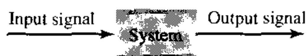
FIGURE 1.1 Block diagram representation of a system.
