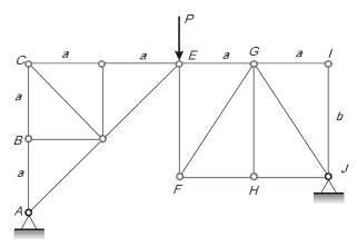
The magnitude (absolute value) of force (in kN) in member *EF* is \_\_\_\_\_\_. (round off to the nearest integer)
