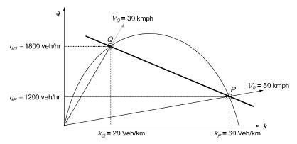
Speed of shock wave (PQ) is, slope of line PQ,
