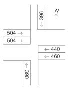
The optimum cycle length (in second), as per the Webster's method, is \_\_\_\_\_\_. (round off to the nearest integer).
