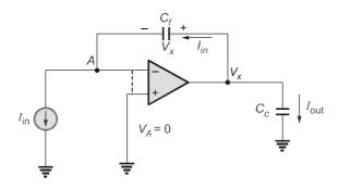
$$V_{x} = \frac{1}{C_{f}} \int I_{in} \times dt = \frac{I_{in}}{C_{f}} \times t$$
