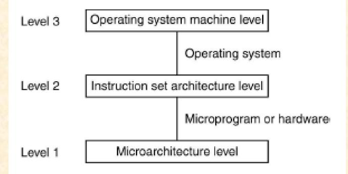
Positioning of the operating system machine level.
