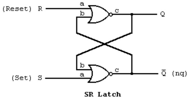
We can specify the same connections that occur in the schematic using VHDL with the following architecture declaration:
