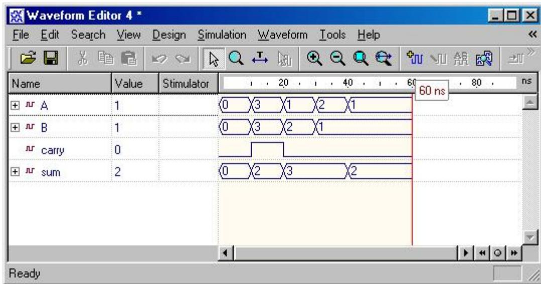
**Write VHDL programs for the comparator, check the waveforms generated.**
