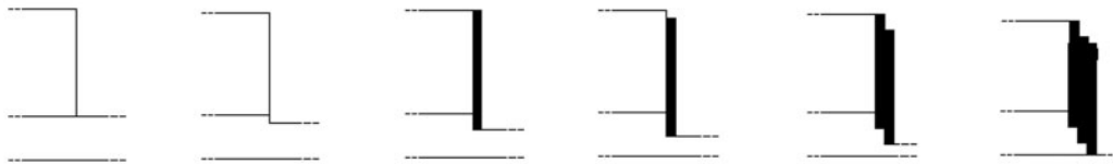
Fig. 21 The sequential formation, from left to right, of an etching feature profile in the presence of redeposition. The etching of horizontal surfaces and redeposition onto vertical surfaces are assumed to occur sequentially.
