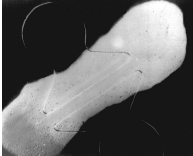
Fig. 4 The first metal-oxide-semiconductor field-effect transistor. 13 (Photograph courtesy of Bell Laboratories, Alcatel-Lucent Co)
