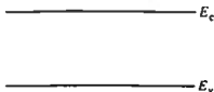
Figure 2.6 The energy band diagram—widely employed simplified version of the energy band model.
