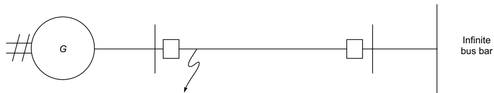
Fig. 8.100 A simple power system
